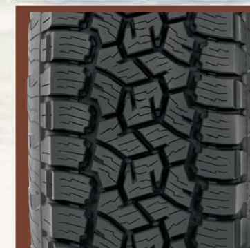
P/Euro-Metric Increased Siping for Wet and Snow Performance
