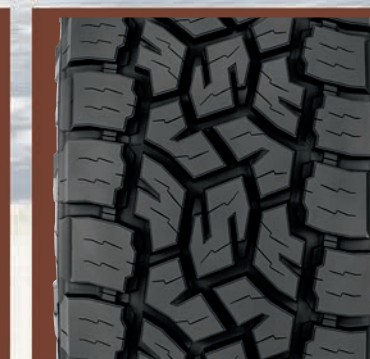
Flotation Larger Tread Blocks and Increased Void
